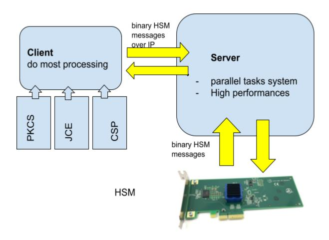
Net Token was a system allowing remote access to an enterprise-grade HSM from a standard PC using a special driver. Locally a PKCS#11 DLL containing all the PKC#11 entry points was present on the PC and under the hood, it was doing remote calls to a PKCS#11 proxy server, handling calls to the HSM. With such a system, access to an HSM could be shared by thousands of customers. A plug-in was developed, cert++, allowing certificates to be also securely remotely stored.
